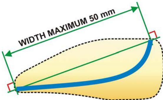
The height of the wing and endplates must not extend higher than the roofline. Wings (excluding endplates) are to be of single molded construction (no flat-packs/bend your own).
